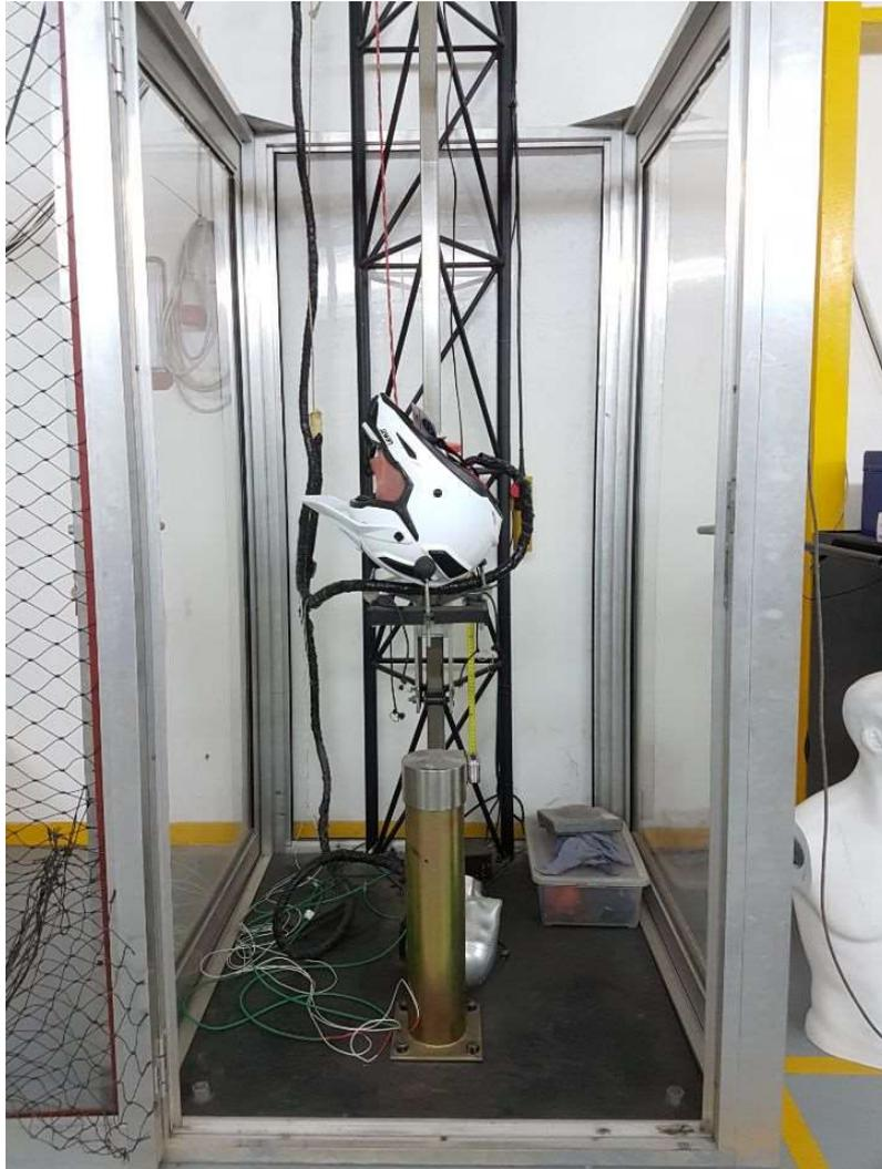
**Figure 4-2: ECE 22.05 test rig**
